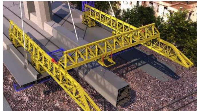
Deck Launching Gantry
